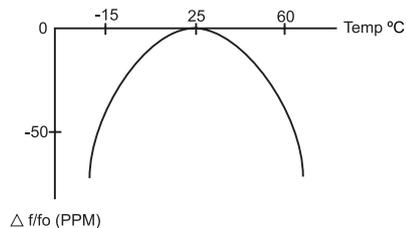
To calculate the frequency stability the parabolic curvature constant (K) is needed.
